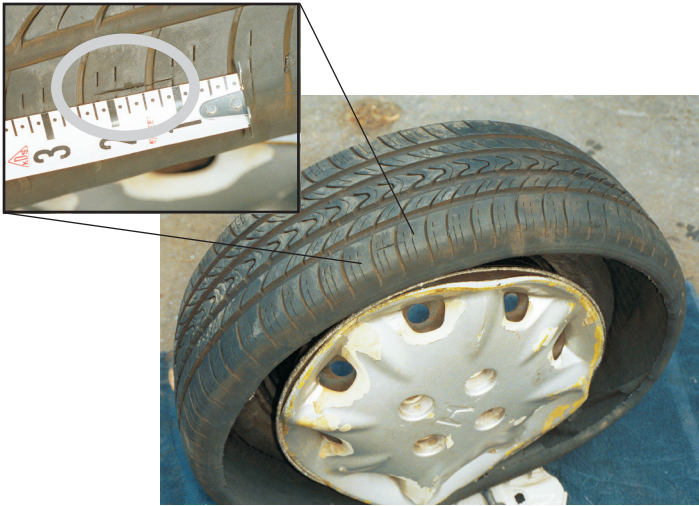
Figure 2. Slash in Tire and Resulting Catastrophic Damage
